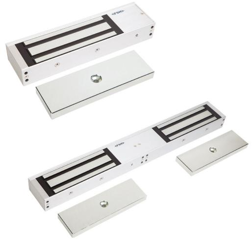
The FEM5700 is an unmonitored single magnetic lock and the FEM5700D is an unmonitored double magnetic lock with dual 12 or 24 Volt settings. The FEM5700M is a monitored single magnetic lock and the FEM5700DM is a monitored double magnetic lock with 12 or 24 Volt settings. Each monitored magnetic lock has a built-in Hall Effect Sensor for remote monitoring of Lock status (LSS).
